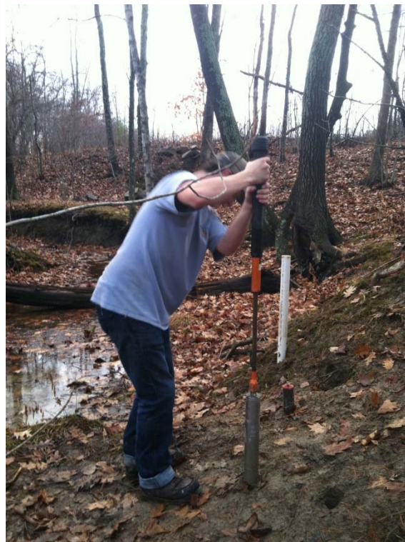
Figure 3: Taking core samples using A) post driver and 2 inch PVC and B) AMS sludge sampler
