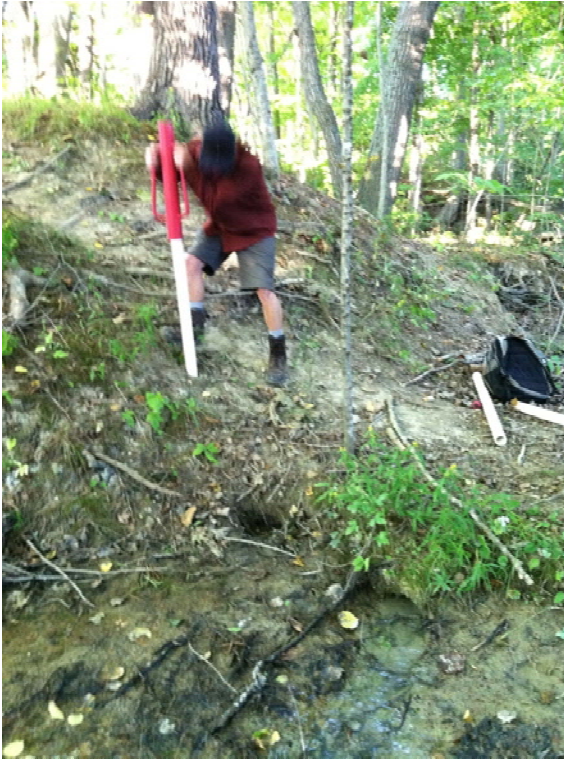
Figure 3: Taking core samples using A) post driver and 2 inch PVC and B) AMS sludge sampler
