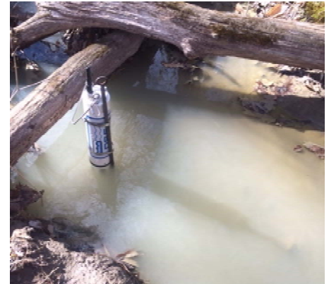
Figure 6: Hydrolab DS-5 in T-Creek. Instrument had protective housing when unsupervised (not shown).
